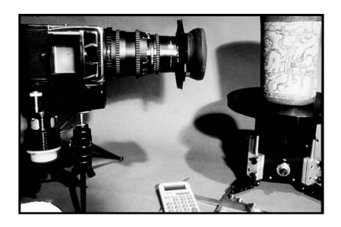
Figure 3 Photograph of equipment employed to create rollout photographs: a Hasselblad camera (modified with addition of continuous motor) and adjustable-speed turntable. The vase atop the turntable is a modern reproduction purchased by the author.
